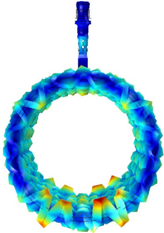
freq(1)=19315 Hz Surface: Total displacement ( \mu\text{m} )
