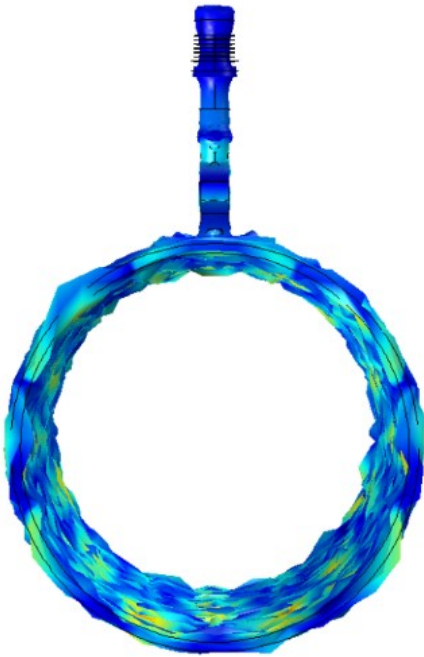
Eigenfrequency=20030 Hz Surface: Total displacement ( \mu\text{m} )
